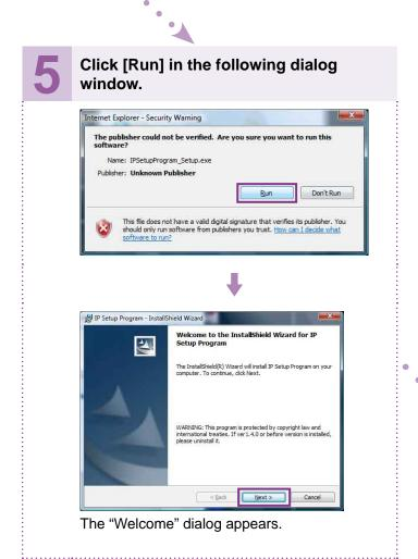
Install the "IP Setup Program" on your computer using the wizard.
